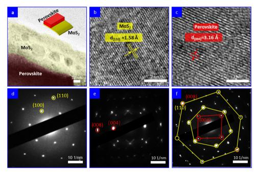
Fig. 2 MAPbI<sub>3</sub> epitaxially grown on  $MoS_2$ . (a) Top-view TEM image of  $MoS_2$  with a MAPbI<sub>3</sub> layer grown on its surface. (b and c) HRTEM images of  $MoS_2$  and  $MAPbI_3$ , respectively. (d and e) SAED patterns of  $MoS_2$  and  $MAPbI_3$ , respectively. (f) SAED pattern of  $MoS_2$  and  $MoS_2$  region, where two distinct diffraction spots can be observed, with the yellow spots representing  $MoS_2$  and the red spots representing  $MoS_3$  and the red
