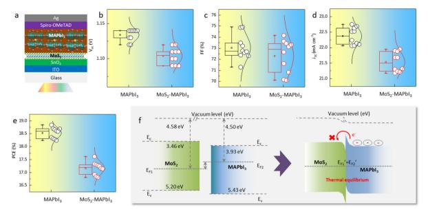
Fig. 4 Bandgap alignment between MoS<sub>2</sub> and MAPbI<sub>3</sub>. (a) Schematic structure of the MoS<sub>2</sub>-MAPbI<sub>3</sub> device. (b–e) Distribution of  $V_{OC}$ ,  $J_{SC}$ , FF, and PCE values collected from 10 MAPbI<sub>3</sub> and 10 MoS<sub>2</sub>-MAPbI<sub>3</sub> devices. (f) Energy level change scheme of MoS<sub>2</sub> and MAPbI<sub>3</sub>.
