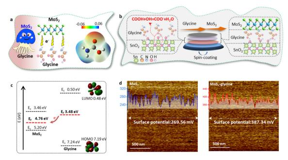
Fig. 5 Formation mechanism of JLMT (a) Jellyfish-like structure consisting of MoS<sub>2</sub> and glycine. (b) Preparation method used to construct the JLMT (c) Electron-transfer scheme between MoS<sub>2</sub> and glycine. (d) KPFM mapping of MoS<sub>2</sub> and MoS<sub>2</sub>-glycine. Inset: CPD profile along the horizontal marked lines.
