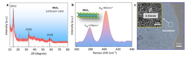
Fig. 1 Properties of the MoS<sub>2</sub> nanosheets. (a) XRD pattern, (b) Raman spectra, and (c) TEM and HRTEM images.
