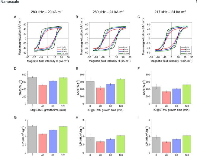
Fig. 10 (A)–(C) Representative hysteresis cycles for the different IO@STMS-t NPs (IO@STMS-0 and for IO@STMS-t (t = 40, 60, 120 min)) obtained from series 2 at different frequency—amplitude conditions. (D)–(F) Corresponding SAR values. (G)–(I). Corresponding ILP values.
