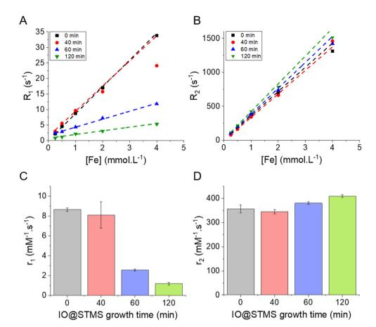
Fig. 9 (A) and (B) respectively the longitudinal  $R_1 = 1/T_1$  (s<sup>-1</sup>) and transverse  $R_2 = 1/T_2$  (s<sup>-1</sup>) relaxation rates as a function of the concentration of iron in the different IO@STMS-t NPs solutions. (C) and (D) respectively the evolution of the longitudinal and transverse relaxivities  $r_1$  and  $r_2$  as a function of the IO@STMS growth time. These results were obtained with the IO@STMS-t obtained from series 2.
