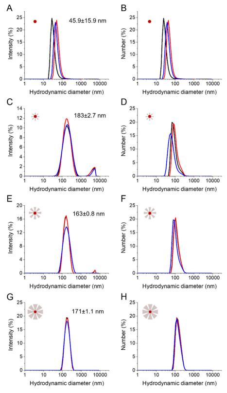
Fig. 8 Colloidal stability in dH<sub>2</sub>O as shown from the distributions of intensity and of the number of hydrodynamic diameters respectively of IO@STMS-0 (A, B), IO@STMS-40 (C, D), IO@STMS-60 (E, F) and IO@STMS-120 (G, H).
