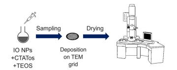
Scheme 2 Schematic representation of the procedure followed to perform the time-lapse TEM imaging.
