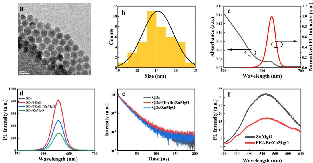
**Fig. 1** The TEM image (a) and size distribution (b) of the QDs. (c) Absorption and PL spectra of the red CdSe/ZnS QDs. (d) The PL of the QDs, QDs/PEABr, QDs/PEABr/ZnMgO, and QDs/ZnMgO deposited on quartz, respectively. (e) TRPL of the QDs, QDs/PEABr/ZnMgO, and QDs/ZnMgO, respectively. (f) PL spectra of ZnMgO and PEABr/ZnMgO.
