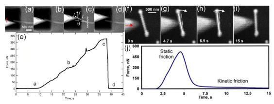
Fig. 17 (a–d) SEM images of the suspended NW being pushed by the tip. (e) The corresponding force curve. Reproduced with permission.<sup>194</sup> Copyright 2011, Elsevier. (f–i) SEM images for the manipulation process of an Ag nanodumbbell. (j) The corresponding recorded tip–nanodumbbell interaction force. Reproduced with permission.<sup>198</sup> Copyright 2015, IOP.
