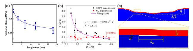
Fig. 31 (a) Frictional shear stress of SiC NWs against the surface roughness of SiN substrate. Reproduced with permission.<sup>222</sup> Copyright 2017, Springer Nature. (b) Dependences of frictional shear stress of ZnO NWs on HOPG and NG substrates on the NW diameter. (c) Sketches of a NW conforming to a wavy substrate surface and the step-induced gap between the NW and substrate surface. Reproduced with permission.<sup>139</sup> Copyright 2022, Springer Nature.
