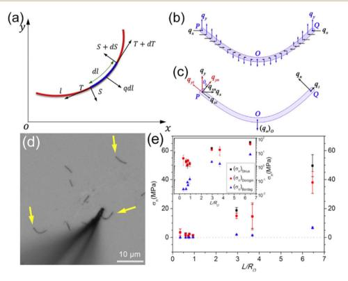
Fig. 22 (a) Schematics of the mechanical model for a bent NW segment held on a substrate by the static friction. (b and c) Distribution of the friction along x and y directions. (d) NWs manipulated to the most-bent state by the W tip under OM. (e) Frictional shear stress calculated by different mechanical models *versus* the  $L/R_{\rm O}$  value. The inset shows the corresponding values in the logarithmic coordinate. Reproduced with permission.<sup>216</sup> Copyright 2015, IOP.
