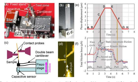
Fig. 19 (a) Experimental setup for the two-manipulator system. (b) Four-legged parallel beam cantilever. (c) Schematic of friction force measurement system. (d) Optical micrograph of two W probes and the targeted Pt wire. (e) The push-pull cycle of the wire against the probes, corresponding to the piezo displacement during friction measurement, and (f) frictional forces recorded at various cycles. Reproduced with permission.<sup>223</sup> Copyright 2011, Elsevier.
