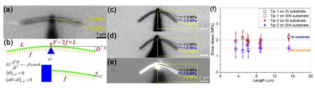
Fig. 23 (a) Optical micrograph of a NW, sliding on the Si substrate at a constant speed due to the push from a W tip. (b) Mechanical loading model for the sliding NW. (c and d) Optical micrographs of the same NW sliding on Si substrate pushed by tip 1 and tip 2, respectively. (e) The same NW to (c and d) slid on SiN substrate pushed by tip 2. (f) Frictional shear stress on Si and SiN substrates plotted as a function of the NW length. Reproduced with permission.<sup>217</sup> Copyright 2015, AIP.
