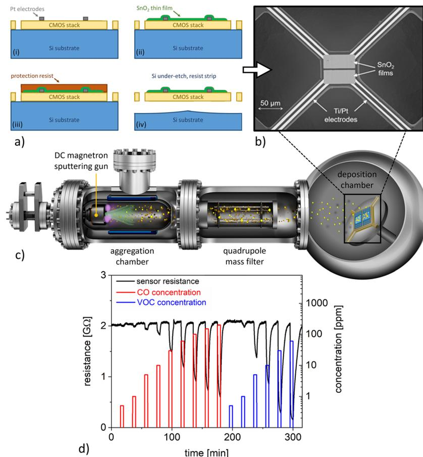
**Fig. 1** (a) Fabrication steps for the realisation of CMOS-integrated SnO<sub>2</sub> thin films sensors. (b) Scanning electron microscopy image of typical device. The sensor structure is integrated on a suspended microhotplate mechanically connected via four arms. (c) Schematic of sensor functionalisation via magnetron-sputtering inert-gas condensation. (d) Chemosensitive signal of a pristine SnO<sub>2</sub>-based gas sensor at 50% relative humidity and an operation temperature of 200 °C.
