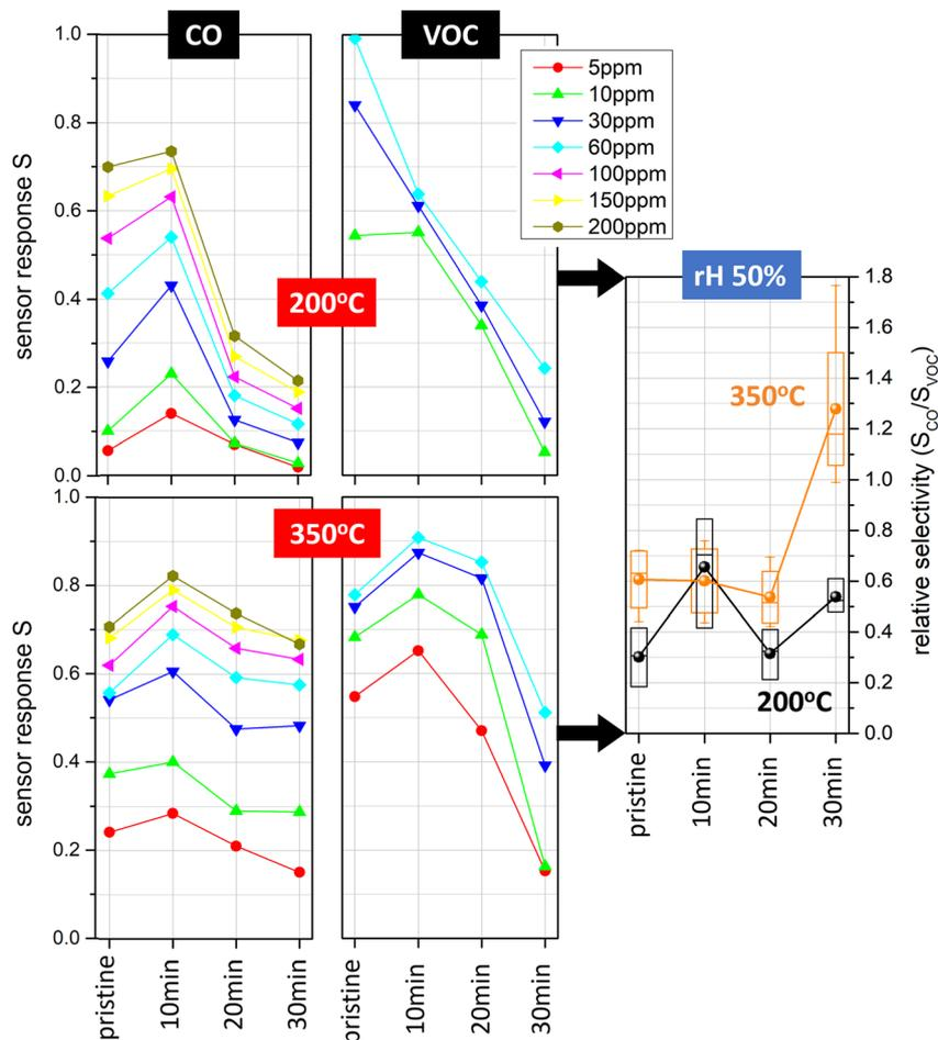
Fig. 4 Sensor response  $S$  to CO (left) and VOC (right) of pristine and Pt-decorated  $\text{SnO}_2$  sensors (nanoparticle deposition times 10 min, 20 min, 30 min) at 50% relative humidity (rH) and operation temperatures of 200 °C (top row) and 350 °C (bottom row). The relative selectivity (averaged in the concentration range 5–60 ppm) of CO response over VOC response is shown in the right graph.
