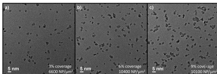
Fig. 3 Low-magnification TEM micrographs of Pt nanoparticles deposited for (a) 10 min, (b) 20 min, and (c) 30 min.
