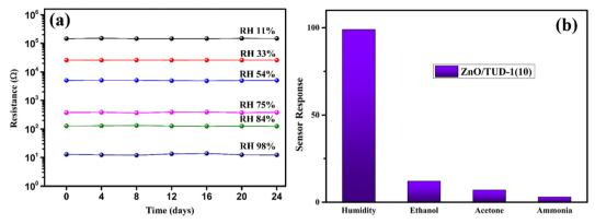
Fig. 11 (a) ZnO/TUD-1(10) sensor showing excellent stability over a time domain and (b) selectivity of the sensor to various gases.
