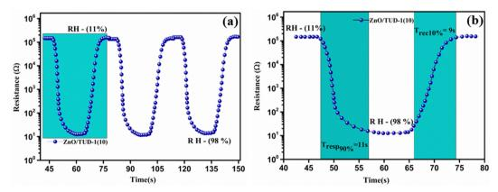
(a) Repeated response and recovery cycles of the ZnO/TUD-1(10) sensor and (b) average response and recovery curve for the ZnO/TUD-1(10) Fig. 10 sensor.
