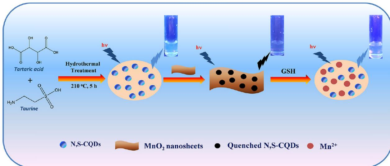
Fig. 7 Schematic representation of designed N,S-CQD-MnO<sub>2</sub> based nanoprobe for the 'off-on' detection of GSH with permission. Copyright 2019, Elsevier.<sup>102</sup>
