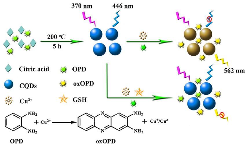
Fig. 8 Schematic illustration of ratiometric FL probe for GSH with permission. Copyright 2019, Elsevier.<sup>127</sup>
