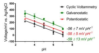
Fig. 3 pH sensitivity of thin, DMSO-treated, wet-spun PEDOT:PSS fibres PANI-coated by CV (10 cycles), potentiostatic (600 s) and galvanostatic (300 s) techniques. The error bars represent the sample stddev of n = 3replicate measurements.
