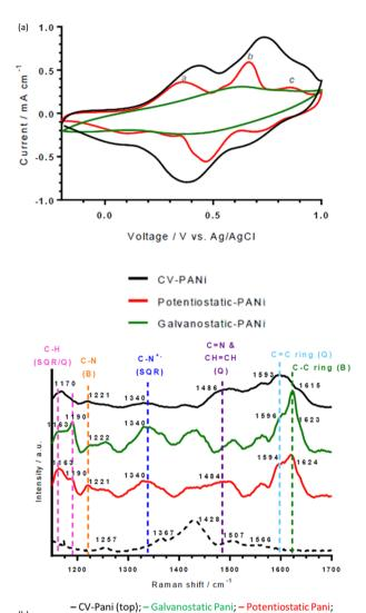
Fig. 1 (a) Cyclic voltammograms and (b) Raman spectra of wet-spun thin, DMSO-treated PEDOT:PSS fibres PANI-coated *via* cyclic voltammetry, potentiostatic and galvanostatic techniques.
