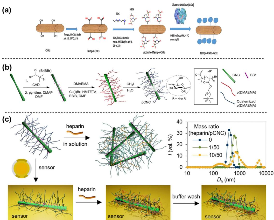
Fig. 13 Applicability of CNCs as biosensors. (a) Schematic representation of CNCs based sensors for glucose sensing,<sup>231</sup> (b) preparation methodology of CNC-based polyelectrolytes,<sup>232</sup> and (c) working mechanism of prepared CNCs polyelectrolytes for heparin sensing and extraction.<sup>232</sup> Reproduced from ref. 231 with permission from Biosensors, MDPI, 2020. Reproduced from ref. 232 with permission from Elsevier, copyright 2021.
