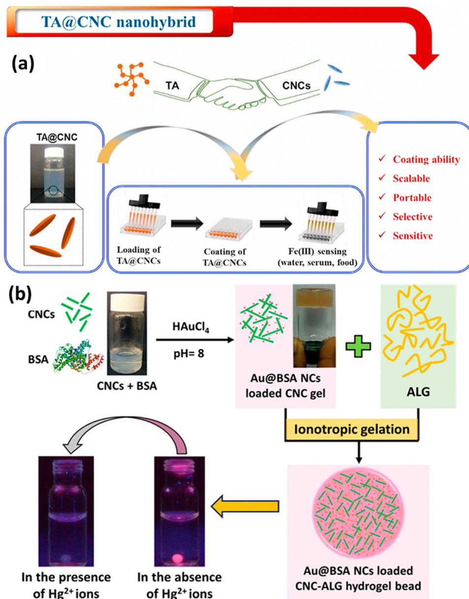
Fig. 5 Use of CNCs in metal sensing: (a) tannic acid loaded CNCs for  $\text{Fe}^{3+}$  detection<sup>161</sup> and (b) bovine serum albumin-protected-gold-nanocluster (Au@BSA NC) loaded CNCs–alginate hydrogel beads.<sup>162</sup> Reproduced from ref. 161 with permission from Elsevier, copyright 2021. Reproduced from ref. 162 with permission from ACS, copyright 2016.
