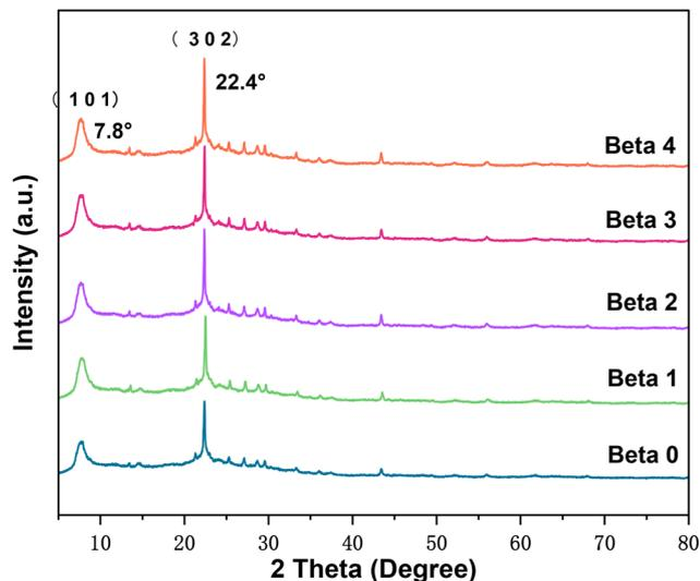
Fig. 4 XRD profiles of all the beta zeolites.
