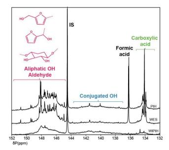
Fig. 6 <sup>31</sup>P NMR spectra of derivatised PIH, WES and WIPIH fractions.
