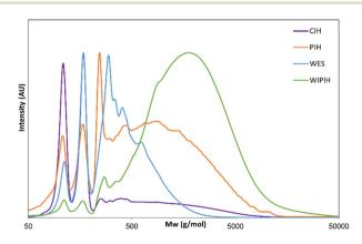
Fig. 3 GPC chromatograms of the different humin fractions measured with the THF method with UV detection.
