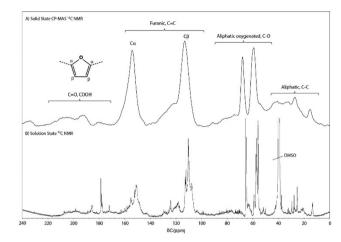
Fig. 4 Solid state CP  $^{13}$ C NMR (A) and solution state  $^{13}$ C NMR (B) spectra of the WIPIH fraction.
