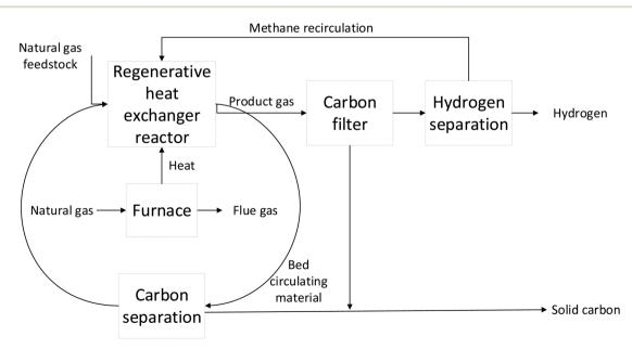
Fig. 4 Turquoise hydrogen (TDM) production (modified from Keipi et al., 2018).<sup>25</sup>
