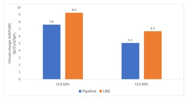
Fig. 10 Blue hydrogen CO<sub>2</sub> capture rate of 60% vs. 90%.
