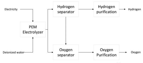
Fig. 5 Overview of green hydrogen (PEM electrolyzer) production (modified from Hermesmann & Müller, 2022). 13,28
