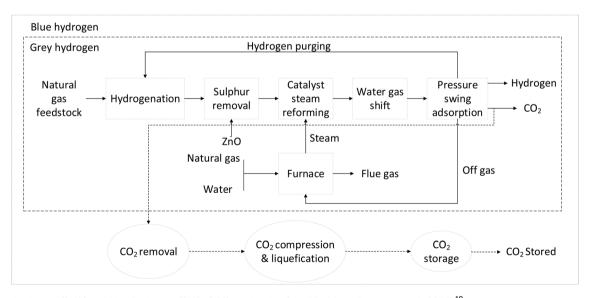
Fig. 3 Grey hydrogen (SMR) and blue hydrogen (SMR-CCS) production (modified from Petrescu et al., 2014).<sup>19</sup>
