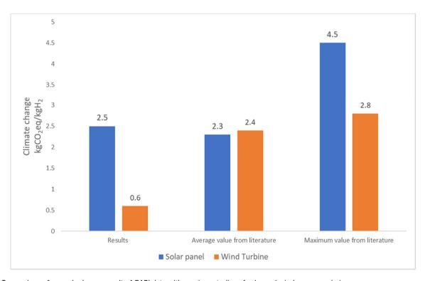
Fig. 12 Comparison of green hydrogen result of GABI data with previous studies of solar and wind energy emission.
