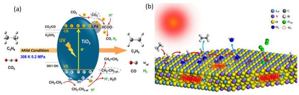
Fig. 17 (a) Schematic representation of (a) photocatalytic oxidative dehydrogenation of  $C_2H_6$  with  $CO_2$  over  $Pd/TiO_2$ ; Reproduced with permission. Copyright 2018, American Chemical Society and (b) photocatalytic  $C_2H_6$  dehydrogenation over  $LaVO_4-O_v$ ; reproduced with permission. Copyright 2024. Elsevier.
