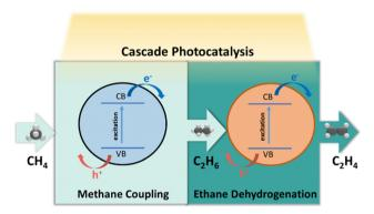
Fig. 16 Schematic representation of the photocatalytic CH<sub>4</sub>-C<sub>2</sub>H<sub>6</sub>-C<sub>2</sub>H<sub>4</sub> cascade system.
