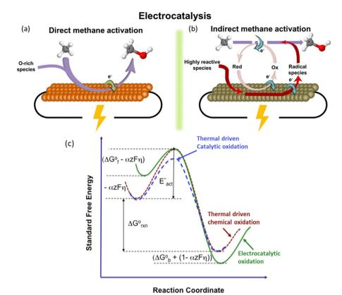
Fig. 4 Schematic illustration of (a) direct electrocatalytic methane activation, and (b) indirect electrocatalytic activation. Reproduced with permission. 15 Copyright 2021, Elsevier. (c) Effects of overpotential on reaction energy profile. Reproduced with permission. 19 Copyright 2016, Elsevier.
