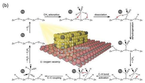
Fig. 14 Schematic representation of photocatalytic NOCM to  $C_2H_4$  reaction mechanisms over (a) Au-Pd/BiNbO<sub>5</sub>F; Reproduced with permission. Copyright 2023, American Chemical Society. (b) AuPd/ZnO. Reproduced with permission. Copyright 2020, American Chemical Society.
