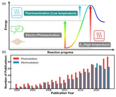
Fig. 2 (a) Energy diagram for low-temperature methane conversion through thermal-, electro- and photocatalysis. Reproduced with permission. Copyright 2019, Elsevier. (b) Number of publications that include "Methane" and "Electro"/"Photo" according to the Web of Science (as on 30 August 2024).
