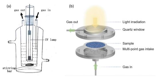
Fig. 15 Schematic representation of photocatalytic methane conversion in (a) batch reactor; reproduced with permission. 71 Copyright 2016, Elsevier. (b) Flow reactor. Reproduced with permission. 104 Copyright 2024, American Chemical Society.
