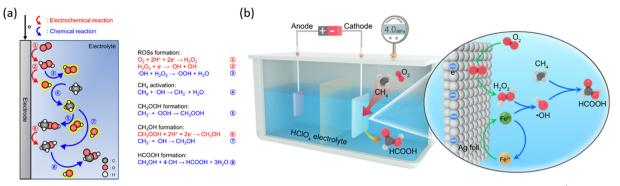
Fig. 7 (a) Schematic illustration of the reaction mechanism for direct POM with the in situ ORR. Reproduced with permission.<sup>48</sup> Copyright 2023, Springer Nature. (b) Schematic illustration of Fenton reaction assisted POM with the in situ ORR. Reproduced with permission.<sup>49</sup> Copyright 2024. American Chemical Society
