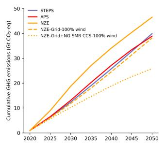
Fig. 6 The cumulative GHG emissions of global H<sub>2</sub> production from 2020 to 2050 in three scenarios
