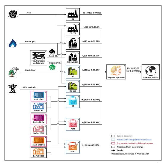
Fig. 1 The LCA model of  $H_2$  production. In this figure, premise is the model of PRospective EnvironMental Impact as SEment. IEA = International Energy Agency database and reports.<sup>2,4,18–20</sup>
