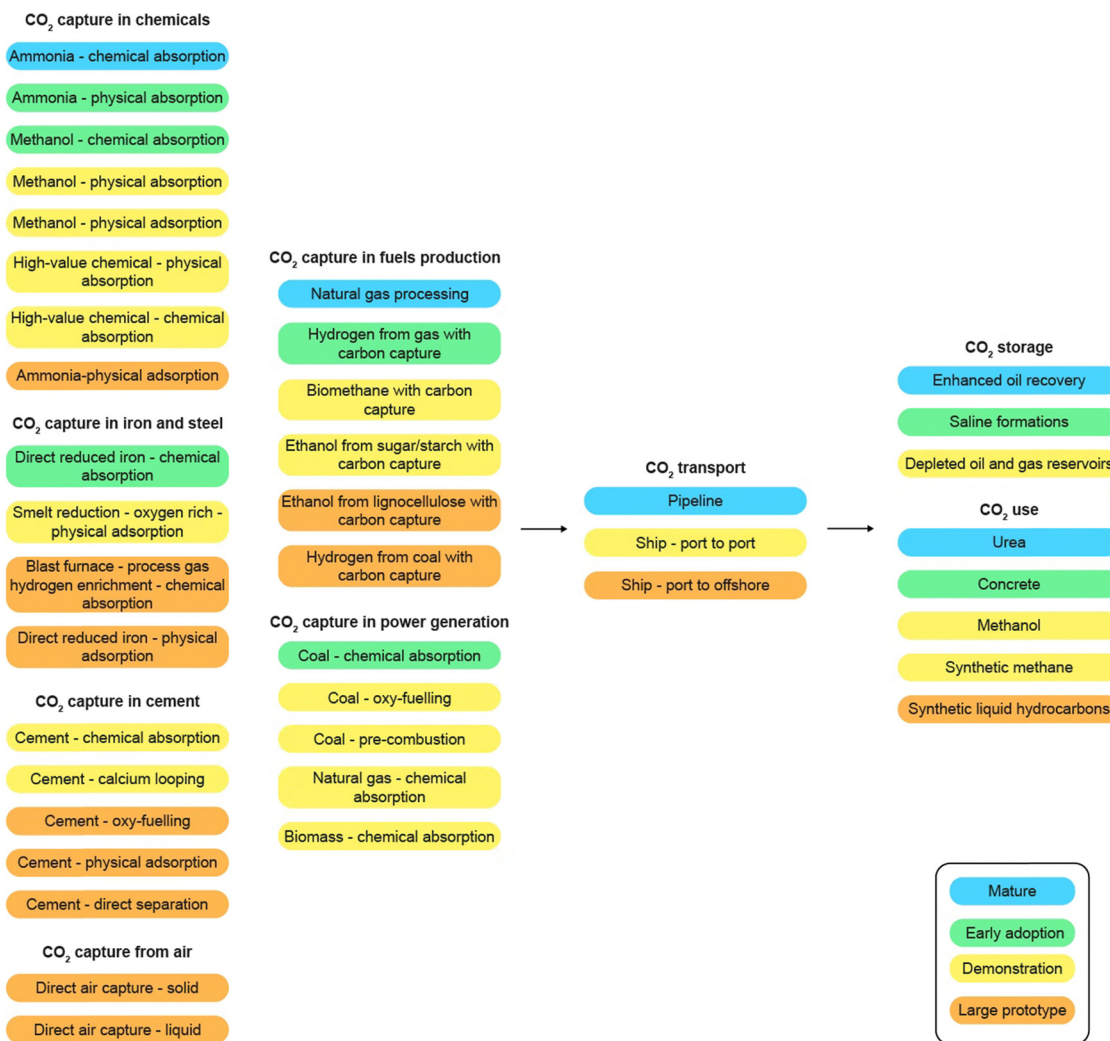
Fig. 4 The technology readiness level (TRL) of multiple technologies along the CCUS value chain. Source, retrieved from ref. 244.
