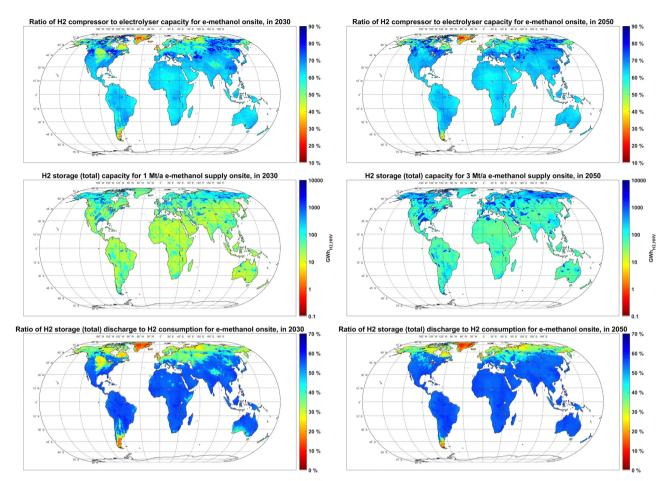
Fig. 10 Relevance of hydrogen balancing technologies, including ratio of H<sub>2</sub> compressor to electrolysers capacity (top), total hydrogen storage capacity (centre), and ratio hydrogen supplied by storage options to the total hydrogen consumption (bottom), in 2030 (left) and 2050 (right).
