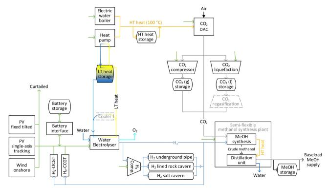
Fig. 1 Power-to-methanol Onsite model configuration. Hydrogen-fuelled gas turbines are considered from 2030 onwards. Abbreviations: H<sub>2</sub>-fuelled open cycle gas turbine (H2-OCGT), H2-fueled combined cycle gas turbine (H2-CCGT), compressor (Comp.), high temperature heat (HT heat), low temperature heat (LT heat), CO<sub>2</sub> direct air capture (DAC), and direct electric heater (DEH)
