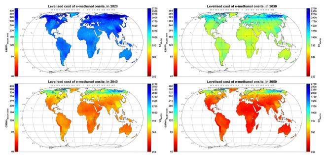
Fig. 4 Levelised cost of e-methanol Onsite in 2020 (top left), 2030 (top right), 2040 (bottom left) and 2050 (bottom right). See Fig. S12 (ESI†) for subfigures with a customised colour bar range for better visualisation of the lowest cost regions at each cost year
