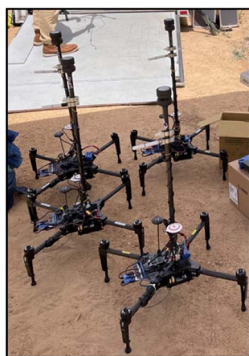
Fig. 9 Four instrumented multirotors used in the campaign.
