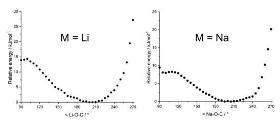
Fig. 7 Potential energy surface scans of the M-O-C angle M-O-C( $CH_2$ ) Ar M=Li-Li left and M=Na-right).
