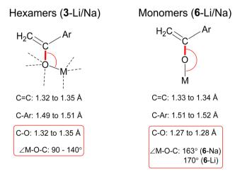
Scheme 4 Comparing the bond lengths in the enolate units of the hexamers and the monomers. The most pronounced structural changes are observed in the C-O bond length and the M-O-C bond angle (highlighted in red).
