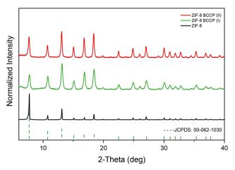
Fig. 1 XRD spectra of non-modified ZIF-8 and BCCP-modified ZIF-8.
