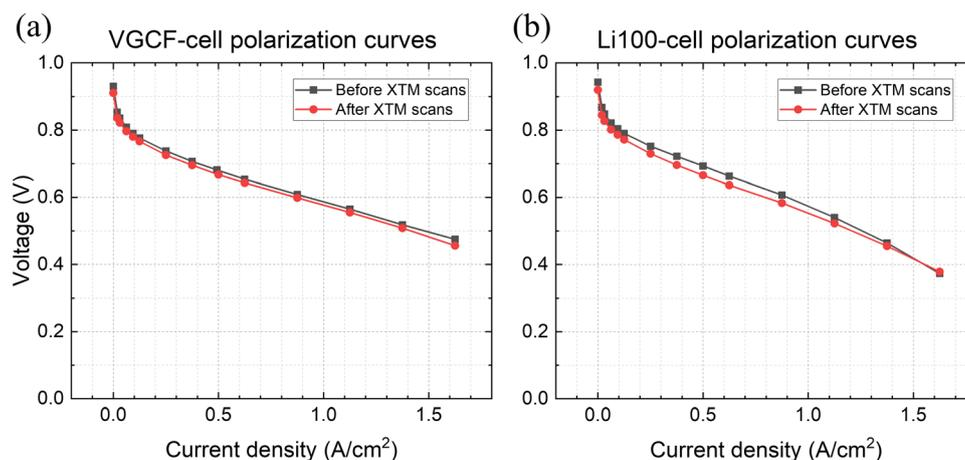
Fig. 2 Polarization curves of (a) VGCF-cell and (b) Li100-cell before X-ray exposure and after all nine tomographic scans; during polarization curve acquisition, cell temperature:  $45 \text{ }^\circ\text{C}$ ,  $\text{H}_2/\text{air}$  flow rate:  $200/200 \text{ mL min}^{-1}$ , relative humidity (RH) of  $\text{H}_2/\text{air}$ :  $100\%/100\%$ .
