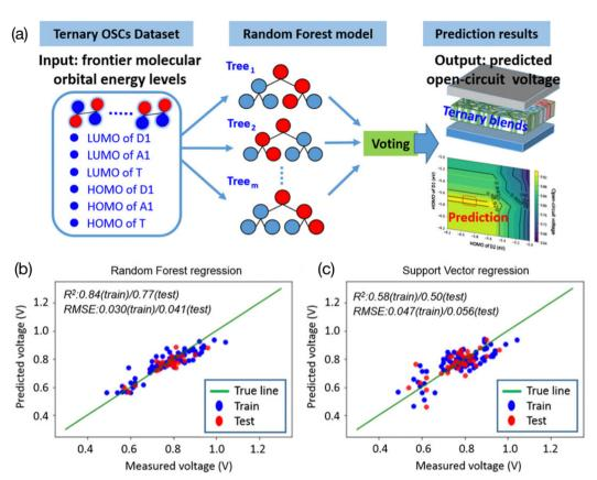
Fig. 4 (a) Using the values of the HOMO and LUMO as features in the ternary OPV  $V_{\rm OC}$  prediction model. (b) The RF model and (c) SVM model. (6) Reproduced from ref. 69 under the terms of the Creative Commons Attribution License from Wiley.
