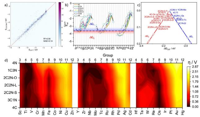
Fig. 10 Taken from Fig. 3 and 4 in Lian et al.<sup>211</sup> (a) DFT calculated and machine learning predicted adsorption energy of Li-polysulfides, (b) predicted adsorption energy of LiS\*, (c) volcano plots for catalysts with an overpotential lower than 0.1 V, and (d) heat map of the predicted overpotential of different SACs. Reproduced with permission.<sup>211</sup> Reprinted (adapted) with permission from ref. 211. Copyright 2021 American Chemical Society.
