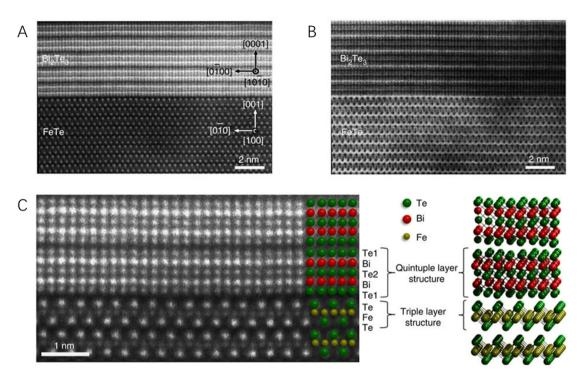
The scanning transmission electron microscopy micrographs of a Bi<sub>2</sub>Te<sub>3</sub>/FeTe heterostructure. (A) The HADDF image. (B) The annular bright field image. (C) The higher-magnification HADDF image showing the atomically sharp interface between Bi<sub>2</sub>Te<sub>3</sub> and FeTe. Reproduced with permission from ref. 75, copyright Springer Nature
