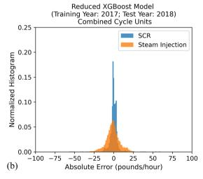
Fig. 6 The distribution of absolute errors, *i.e.*, the difference between the predicted  $NO_x$  emission rates and the CAMD-derived  $NO_x$  emission rates, for the combined cycle units with different  $NO_x$  control technologies (with SCR, steam injection) output from the (a) full XGBoost model; (b) reduced XGBoost model trained on 2017 data and tested on 2018 data.
