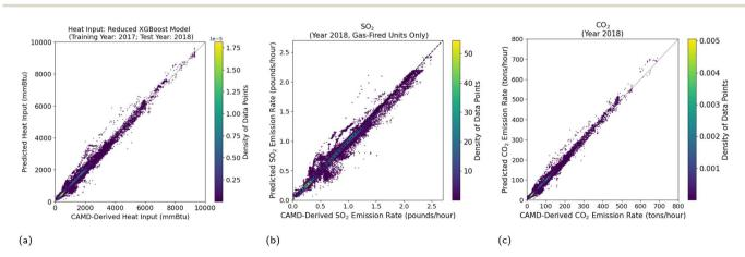
Fig. 9 The scatter plot of (a) measured *versus* predicted hourly heat input from the reduced XGBoost model (trained on 2017 data and tested on 2018 data); (b) CAMD-derived *versus* predicted SO<sub>2</sub> emission rates for gas-fired hours only, with the predicted values calculated by eqn (3) using the predicted hourly heat input; (c) CAMD-derived *versus* predicted CO<sub>2</sub> emission rates, with the predicted values calculated by eqn (4) using the predicted hourly heat input.
