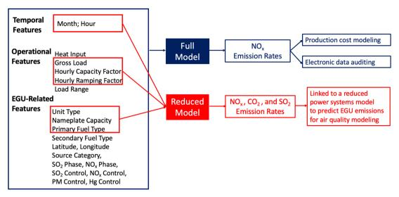
Fig. 3 Two distinct ML-based models, full model, and reduced model, for different applications
