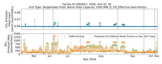
Fig. 8 The ratios between  $CO_2$  emissions and heat input (upper), and CAMD-derived *versus* predicted  $NO_x$  emission rates (bottom,  $R^2 = 0.88$ ) from Unit 30 of the Ravenswood Generating Station facility in Long Island City, NY (Facility ID: 2500) in 2018, with  $NO_x$  emission rates of about 160 data points over-predicted in June, July, August and September corresponded with the over-prediction zone shown in the left scatter plot in Fig. 5a.
