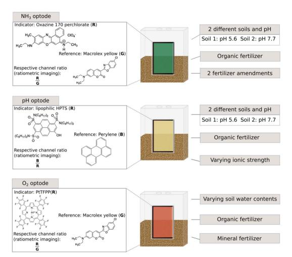
Fig. 1 Overview of the experimental set-up and utilised optodes as well as the various test scenarios, pH values were measured with a pH electrode.
