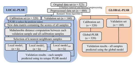
Fig. 3 Flow chart of LOCAL-PLSR and GLOBAL-PLSR calibration procedures. For a given sample in the validation set, *k* is the number of nearest neighbor samples selected in the calibration set considering a given Mahalanobis limit distance.
