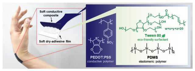
Fig. 1 Optical and schematic images of the skin-adherable soft strain sensor featuring a bilayer architecture composed of a soft conductive composite and a soft dry-adhesive film, along with the molecular structures of the individual components
