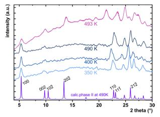
Fig. 12 High-temperature PXRD of PTCDI-Ph (phase II at 350, 400 and 490 K and phase I at 493 K) measured with Cu K $\alpha$ , and the pattern at the bottom with indicated hkl planes is the calculated diffractogram from the single-crystal measurements collected at 490 K.
