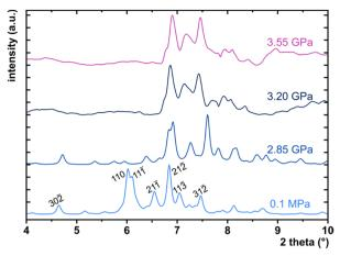
Fig. 11 PXRD collected for PTCDI-Ph phase II at 0.1 MPa, 2.85 and 3.20 GPa as well as phase III at 3.55 GPa. The measurements were performed using synchrotron X-ray diffraction ( $\lambda = 0.4099$  Å). Patterns for 0.1 MPa and 2.85 GPa are the calculated diffractograms from singlecrystal measurements
