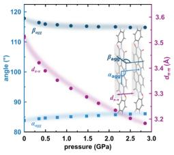
Fig. 7 Changes in the packing of PTCDI-Ph phase II under compression (b): purple circles mark the distance between  $\pi$ -stacked molecules ( $d_{\pi-\pi}$ ) and blue symbols represent the packing angles  $\alpha_{aqq}$  and  $\beta_{aqq}$  (cf. Fig. 4).
