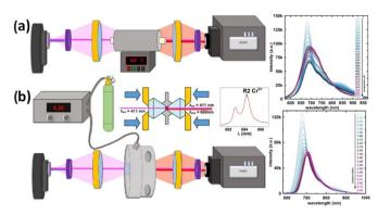
Fig. 10 Schematic drawings of experimental setups with PTCDI-Ph crystals applied as (a) high-temperature and (b) high-pressure sensors. The accompanying plots illustrate the shifts in the respective luminescence spectra (cf. Fig. 5 and 9).
