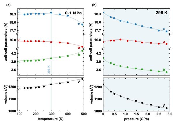
Fig. 3 Temperature (a) and pressure (b) dependence of the unit-cell dimensions a, b, c (top) and its volume (bottom) for PTCDI-Ph phase II. Open symbols mark the data previously reported by Sato and Mizuguchi. 38 The estimated standard deviations (ESDs) are smaller than plotted symbols. The blue highlight indicate the data measured at 296 K. The changes in monoclinic angle  $\beta$  are shown in Fig. S5 in the ESI.†
