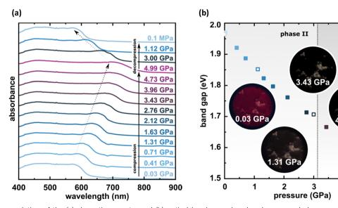
Fig. 8 Pressure evolution of the (a) absorption spectra and (b) optical band gap; closed and open symbols correspond to the compression and decompression runs, respectively. The inserted photos show the PTCDI-Ph film prepared for measurements of UV-vis spectra at 0.03, 1.31, 3.43 and 4.99 GPa, showing the darkening of the sample as the pressure increases.
