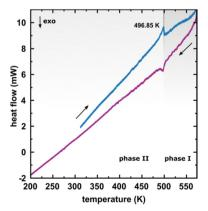
Fig. 6 Differential scanning calorimetry (DSC) thermogram of PTCDI-Ph in the heating and cooling cycles.
