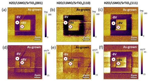
Fig. 3 (a-c) PFM out-of-plane phase images for the three HZO films grown on LSMO/SrTiO<sub>3</sub>(001), LSMO/SrTiO<sub>3</sub>(110), and LSMO/SrTiO<sub>3</sub>(111), respectively, after applying +(-)8 V in the bright (dark) regions. The outer region corresponds to the as-grown state and no voltage has been applied. (d-f) PFM out-of-plane amplitude images corresponding to the (a-c) phase image regions.
