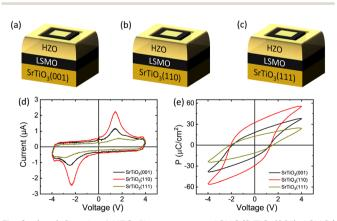
Fig. 2 (a-c) Sketch of HZO films grown on LSMO/SrTiO<sub>3</sub>(001), LSMO/ SrTiO<sub>3</sub>(110), and LSMO/SrTiO<sub>3</sub>(111), respectively. (d and e) Corresponding I-V and P-V loops measured at 1 kHz for the three samples.
