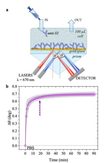
Fig. 1 (a) Schematic representation of the SPR Navi 200-L apparatus in the Kretschmann configuration. The manual injection of a sample volume of 100 µL is performed with a sterile syringe. (b) The open symbols refer to the sensogram ( $\Delta\theta$  vs. time) registered during the physisorption of anti-S1 on the SPR gold slide. The solid line is fitted with eqn (1). The purple dotted arrow indicates the minimum time required for the biolayer to reach 95% surface coverage, namely 19 minutes.
