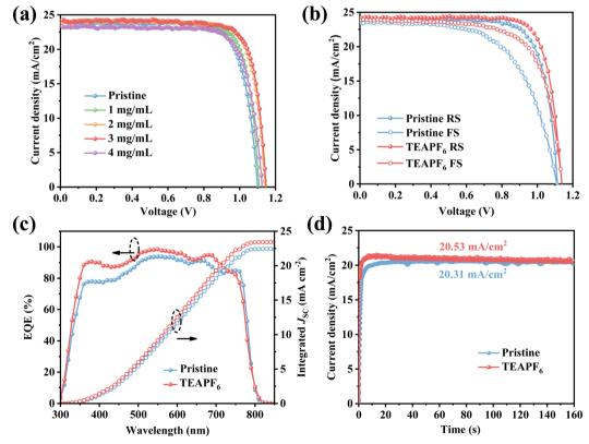
Fig. 3 (a) J-V curves of PSCs with different concentrations of TEAPF<sub>6</sub>. (b) J-V curves in different scan directions. (c) EQE spectra and (d) steady-state output  $J_{SC}$  of PSCs.
