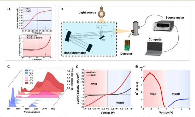
Fig. 2 Performance of dual-band visible and SWIR photodetectors. (a) Current density-voltage curves of CdTe/ZnO single-band device and ZnO/HgTe/ Ag<sub>2</sub>Te single-band device. (b) Illustration of the performance characterization system. (c) Response spectra of the dual-band device under positive and negative bias. (d) Current density-voltage curves of the dual-band device. (e) Specific detectivity of the dual-band device under positive and negative bias
