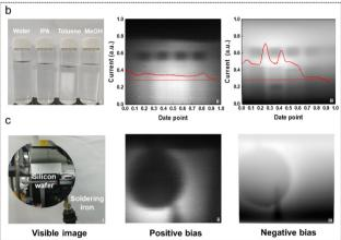
**Fig. 4** Dual-band imaging. (a) Illustration of the single-pixel scanning imaging setup. (b) and (c) Visible images (i) and the images captured by the dual-band detector under positive (ii) and negative (iii) bias voltages for (b) four different chemical solvents in glass vials and (c) a silicon wafer and soldering iron arrangement.
