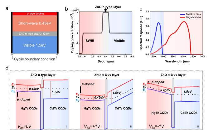
Fig. 3 Simulation of the dual-band visible and SWIR photodetector. (a) Simulation model structure of the dual-band device. (b) Distribution of the doping concentration. (c) Simulated spectral responses of the dual-band device under negative and positive bias voltages. (d) Simulated energy band diagram of the dual-band device under zero (i), positive (ii), and negative (iii) bias voltages.
