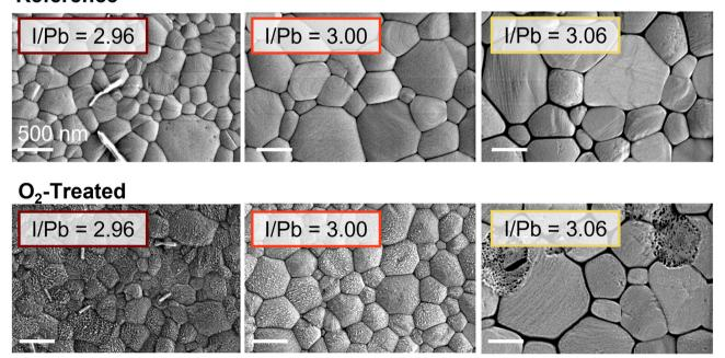
Fig. 2 Representative SEM images of reference and oxygen-treated glass/ITO/PEDOT:PSS/Perovskite films for the understoichiometric, stoichiometric, and overstoichiometric cases
