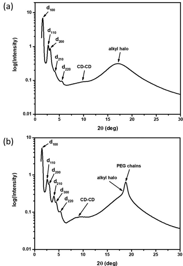
Fig. 4 X-Ray diffractograms of 2 at (a) 95 °C ( $Col_h$ ) and (b) room temperature ( $Col_h^*$ ).
