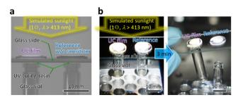
Fig. 4 (a) Schematic and (b) results of the demonstration of a utility of the UV-UC film applied to a solidification of UV curing resin with visible light ( $\lambda > 413$  nm) of 1  $\odot$  intensity at the sample position. Samples used here did not have a reflection aluminum layer on the bottom side.
