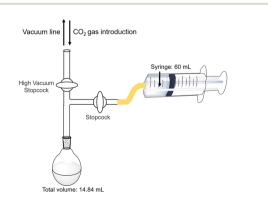
Fig. 4 Outline of the experimental setup for the estimation of the amount of CO<sub>2</sub> in the gas phase captured in a sample solution.
