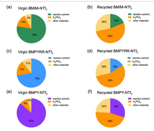
Fig. 4 Contribution of major cost drivers resulting from Pt nanoparticle syntheses using virgin and recycled (a and b) BMIM-NTf<sub>2</sub>, (c and d) BMPYRR-NTf<sub>2</sub>, and (e and f) BMPY-NTf<sub>2</sub>, respectively.
