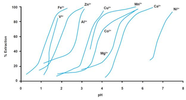
Fig. 9 Extraction equilibria of metals (in%) using cyanex 272 vs. pH in sulphate solutions (reproduced from ref. 43 with permission from KISTI, copyright 2015).
