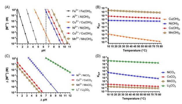
Fig. 8 Solubility diagram for metal hydroxides at 25 °C (A) temperature effect on metal hydroxide solubility (B) solubility diagram for metal carbonates at 25 °C (C) and temperature effect on metal carbonate solubility (D) (reproduced from ref. 30 with permission from ACS, copyright 2022).
