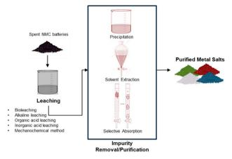
Fig. 5 Recycling using hydrometallurgical processing
