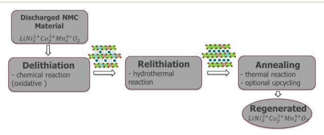
Fig. 15 Typical direct recycling process for NMC cathodes.
