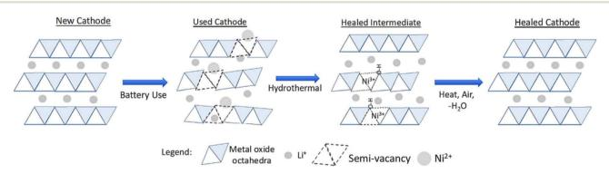
Fig. 17 OnTo technology's advanced battery recycling process for LIBs: cathode-healing™ impacts structure by mixing Ni<sup>2+</sup> and Li<sup>+</sup> to regenerate the full layered structure (reproduced from ref. 64 with permission from Elsevier, copyright 2019).
