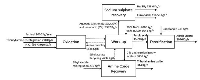
Fig. 4 Process scheme showing different sections of the process with mass balance
