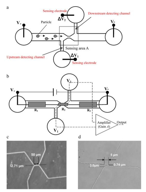
Fig. 4 (a) Representation of a microfluidic setup for the detection of nanoparticles (b) circuit model of the sensor, (c) detection of 490 nm sized nanoparticle, and (d) detection of 220 nm sized nanoparticle.80
