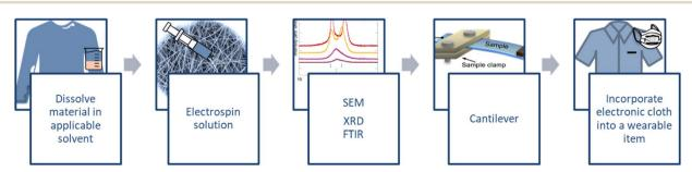
Fig. 2 A schematic illustrating the proposed end-of-life process for repurposing piezoelectric materials including synthesis, characterization, and possible outcome.
