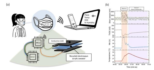
Fig. 6 (a) Conceptual schematic illustrating the potential application and implementation of recycled acrylic materials for piezoelectric sensing. (b) Raw data from a one-minute use of a clothe mask outfitted with the electronic textile made from recycled acrylic sweater and a Bosch RMF680 sensor
