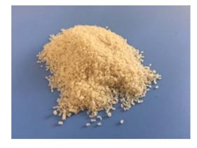
Fig. 10 PLA-based 100% biomass biodegradable plastic for injection, biaxial stretch blow molding.<sup>59</sup>
