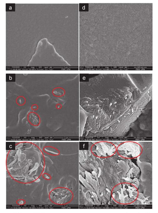
Fig. 12 FESEM images at 500 00× and 1 000 00× magnification of the fractured surfaces of neat PLA (a and d), PLA/CNF3 (b and e), and PLA/ CNF6 (c and f), respectively. Red circles show nanocellulose. PLA/CNF6 exhibits agglomerated nanocellulose. CNF: nanocellulose. Number after CNF indicates the % against the weight of PLA.60
