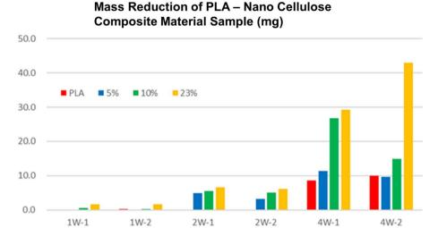
Fig. 4 Biodegradability test result. It can be seen that biodegradability increased as the content of nanocellulose increases in the PLA-nanocellulose composite material.49
