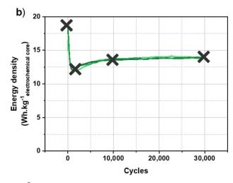
Fig. 5 Long-term cycling of a hybrid KIC in 0.8 mol  $L^{-1}$  KPF<sub>6</sub> AN at 16 mA cm<sup>-2</sup> between 0.5 and 3.5 V at room temperature in the pouch cell configuration after CC formation (a) and after CV formation (b).8
