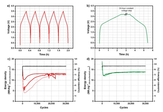
Fig. 1 Voltage profiles at room temperature during CC formation (a) and CV formation (b) and energy densities and coulombic efficiency during long-term cycling at 16 mA cm<sup>-2</sup> between 0.5 and 3.5 V in the pouch cell configuration after CC formation (c) and CV formation (d).
