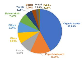
Fig. 2 Average composition of the rest fraction of MSW in Spain. Source: PFMAR 2016-2022 58
