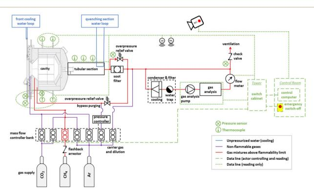
Fig. 4 Experimental setup at the solar tower of IMDEA Energy, depicting the solar reactor, the feeding and handling of reactant gases, and the measurement instrumentation.
