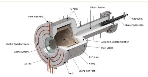
Fig. 1 Solar reactor configuration, consisting of a cavity-receiver with a windowed aperture containing a reticulated porous ceramic (RPC) structure made of ceria.
