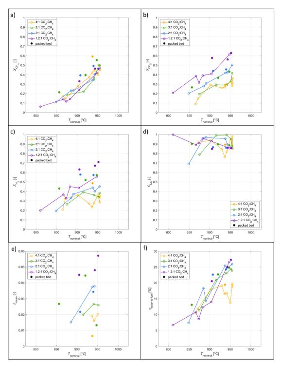
Fig. 9 Experimental results as a function of the nominal temperatures for the co-feeding runs: (a) CH<sub>4</sub> molar conversion. (b) CO<sub>2</sub> molar conversion. (c) H<sub>2</sub> selectivity. (d) CO selectivity. (e) Average  $\delta$  of CeO<sub>2- $\delta$ </sub>. (f) Solar-to-fuel energy efficiency. Tests were performed at varying inlet  $CO_2$ :  $CH_4$  (3:1, 3:1, 2:1, 1.2:1) 40% diluted in Ar, and with the packed bed installation in the tubular section.
