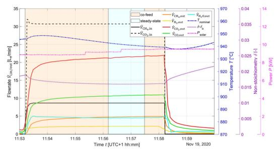
Fig. 8 Solar radiative power input, nominal temperature, inlet/outlet gas compositions, and  $\delta$  of CeO<sub>2- $\delta$ </sub> as a function of time for the co-feeding run. Flowrate data was smoothed using a local regression with weighted linear least squares and a 2nd degree polynomial.  $H_2O$  flow rate data was determined via C: H ratio balance
