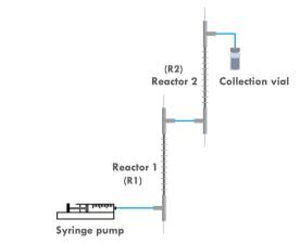
Fig. 3 Scheme of the two-reactor setup.
