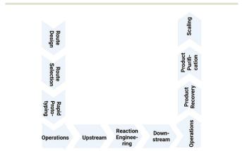
Fig. 1 Workflow for metabolite synthesis from route design and selection, rapid prototyping, reaction engineering, upstream and downstream operations, product recovery and purification to scaling.
