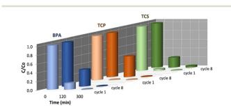
Fig. 5 Different results in BPA, TCP and TCS removal at 120 and 300 min. Comparison between the first and eighth cycle of HY-AC-SBP treatment.
