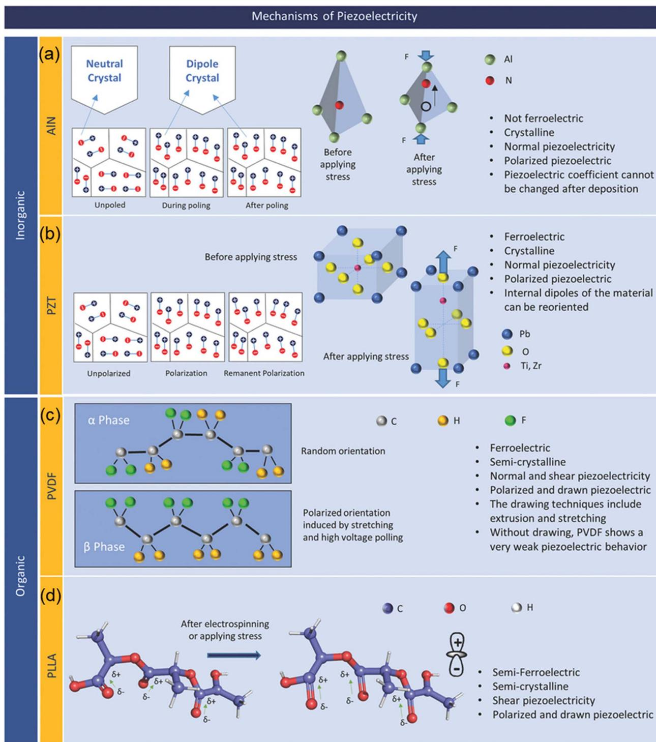
Fig. 2 Representative piezoelectric materials and their mechanisms: (a) AIN; (b) PZT; (c) PVDF; and (d) PLLA. Reproduced with permission from ref. 32 Copyright 2019 John Wiley and Sons.
