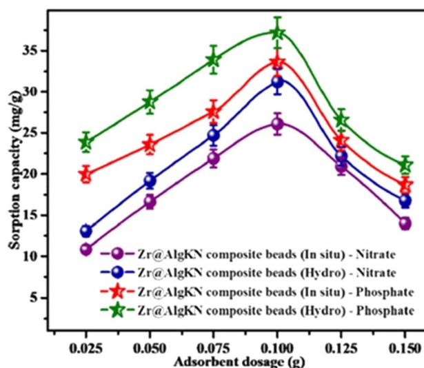
Fig. 5 Effect of adsorbent dose on adsorption capacity of *in situ* and hydrothermal synthesized Zr@AlgKN composite beads towards  $\text{NO}_3^-$  and  $\text{PO}_4^{3-}$ . Reproduced with permission from ref. 86 with permission from Elsevier, copyright 2020.
