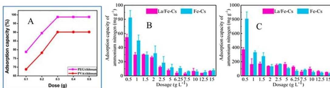
Fig. 10 (A) The effect of PEG/chitosan and PVA/chitosan composite dose on  $\text{NO}_3^-$  adsorption<sup>101</sup> with permission from Elsevier, copyright 2016. (B) The effect of Fe-Cs and La/Fe-Cs composite dose on ammonium-nitrogen removal from cow breeding wastewater and (C) pig farm wastewater. Reproduced with permission from ref. 1 with permission from Elsevier, copyright 2022.
