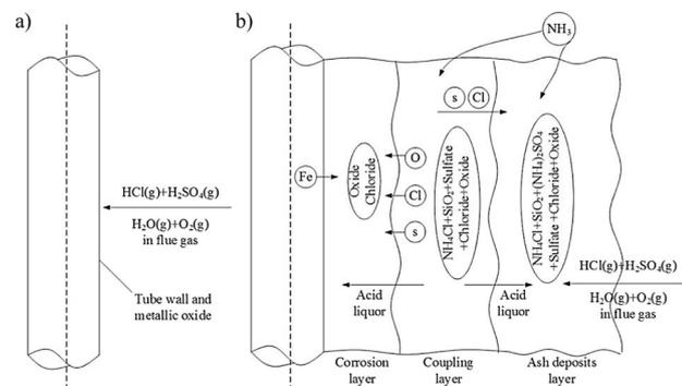
Fig. 10 Schematic of dew point corrosion process. (a) The first stage. (b) The second stage.<sup>179</sup>
