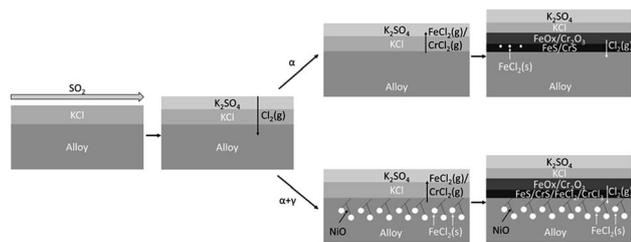
Fig. 5 Schematic overview of the proposed corrosion mechanism depending on the microstructure.<sup>133</sup>
