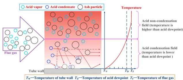
Fig. 9 Coupling model of acid condensation and fly ash.<sup>178</sup>
