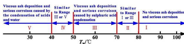
Fig. 8 Ash deposition and corrosion characteristics as a function of wall temperatures.<sup>173</sup>
