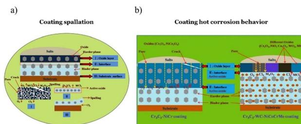
Fig. 7 Schematic diagram of deposit induced hot corrosion mechanisms on NiCr base coating, (a) Cr<sub>3</sub>C<sub>2</sub>-NiCr coating spallation mechanisms<sup>170</sup> and (b) hot corrosion behavior of Cr<sub>3</sub>C<sub>2</sub>-NiCr and Cr<sub>3</sub>C<sub>2</sub>-WC-NiCoCrMo coating.<sup>174</sup>
